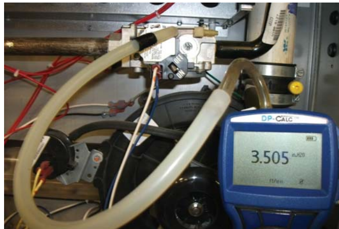
FIGURE 30 - MANOMETER MEASURING GAS MANIFOLD PRESSURE
